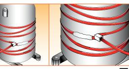
Thermwire-Comp heaters are used to prevent migration of refrigerant into crankcase oil when compressors are operated in cold temperatures. Use of these heaters can prevent excessive wear and loss of refrigerant efficiency.
