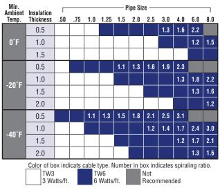
Note: TW3 is UL Listed for metal and plastic pipes. TW6 is UL listed for metal pipe only.
