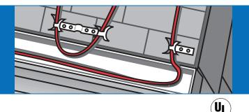
Thermwire-Melt prevents costly structural damage to roofs, gutters and downspouts caused by ice and snow. Apply anywhere melting snow and ice can penetrate roof surface and refreeze, lifting shingles, pulling gutters away, and breaking gutters and downspouts.
