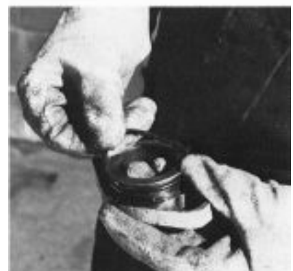
REPLACING GLAND O-RINGS
