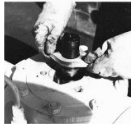
PACKING GLAND REMOVAL
