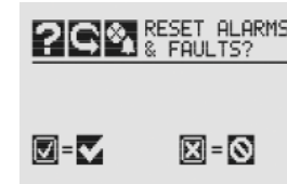
Figure 21. Alarm/Fault Reset Confirmation Screen
