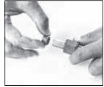
Step 2 – Slip nut and ferrule over deburred tube end. Be sure the long, straight end of the ferrule points toward tube end.
