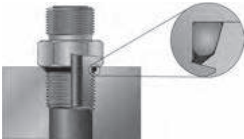
Fig. R1 – SAE / ISO / JIS B2351 Straight Thread Port O-Ring Upon Assembly
