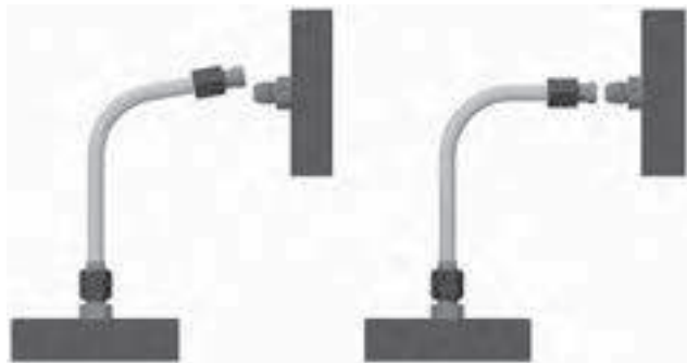
Fig. R33 – Improper bend and short tube
