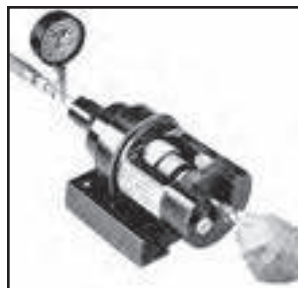
Fig. R29 — Flaring with Hydra-Tool
