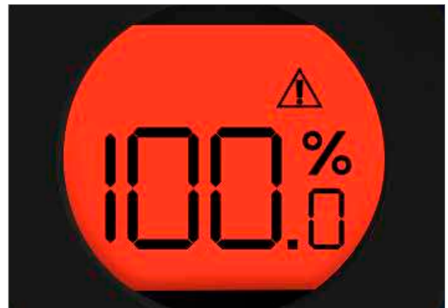
Fig 4.7 Actuator flashes Red and White alternatively when power failure occurs
