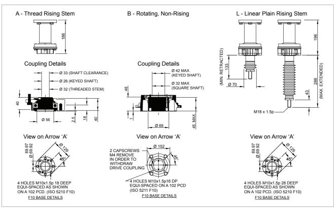
Note: A and B couplings are removable and supplied blank for machining. For full detailed drawings visit www.rotork.com
